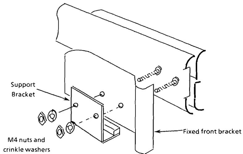
**Fig. 2.5 Fitting a front bracket and support bracket**
