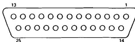
**Fig 1.1** Multi-Channel Connector
