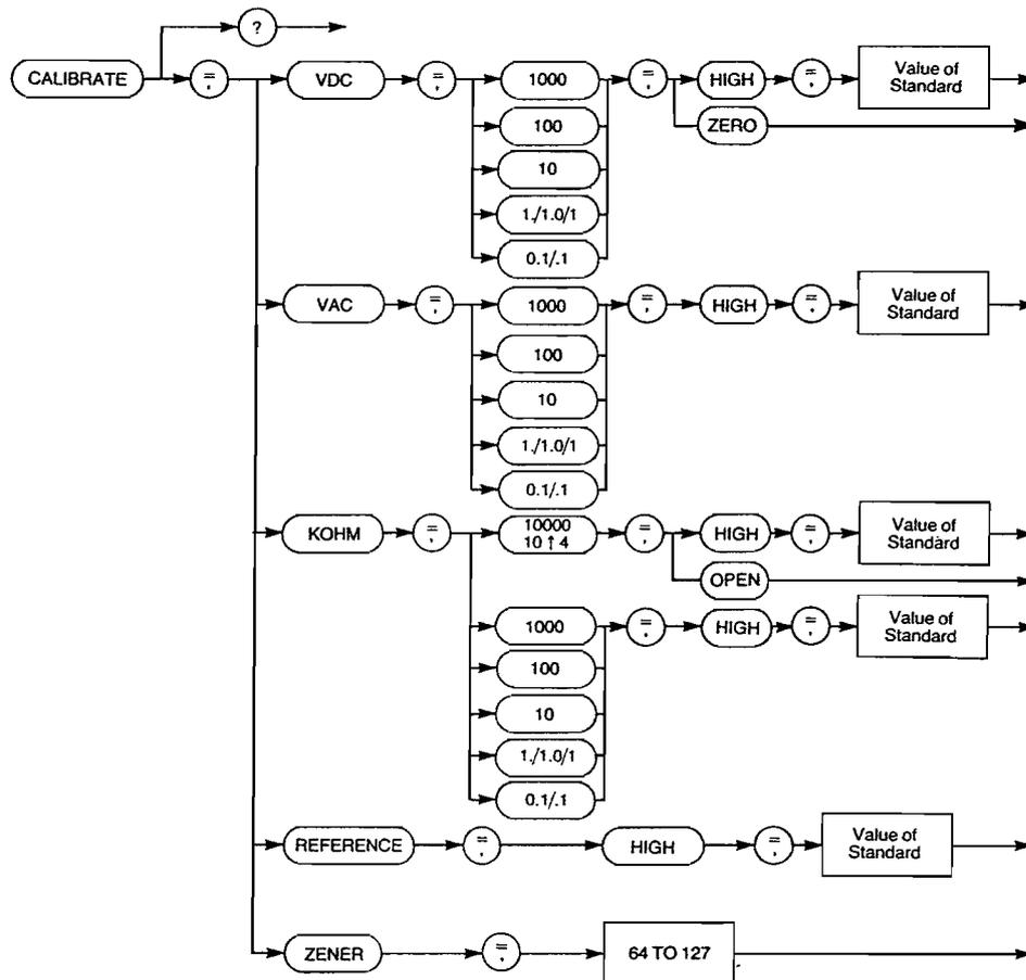
**Fig 3.3** Calibrate Command
