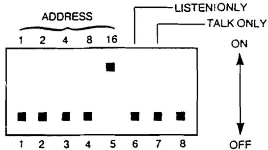
Fig 1.4 GP-1B Selector Switches
