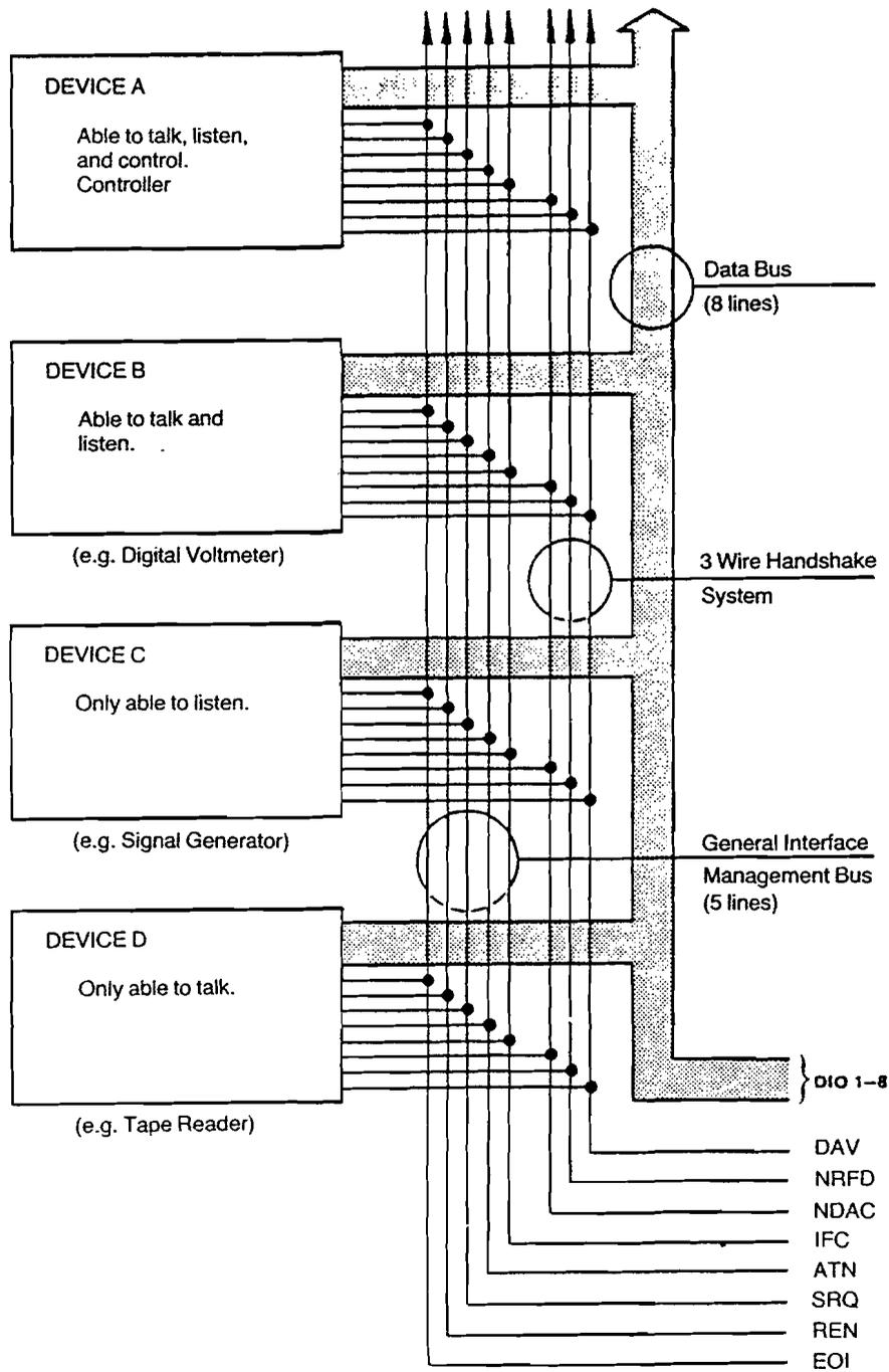
Fig 1.2 GP-IB Structure
