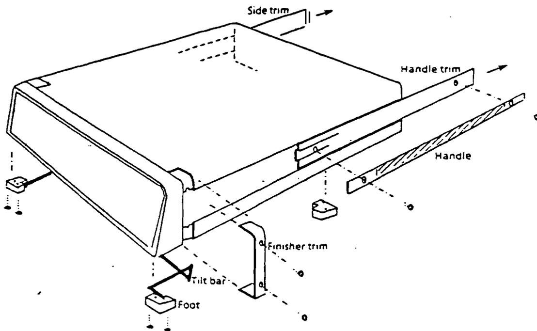
Fig. 2.1 Removal of trims, handle, feet and tilt bar
