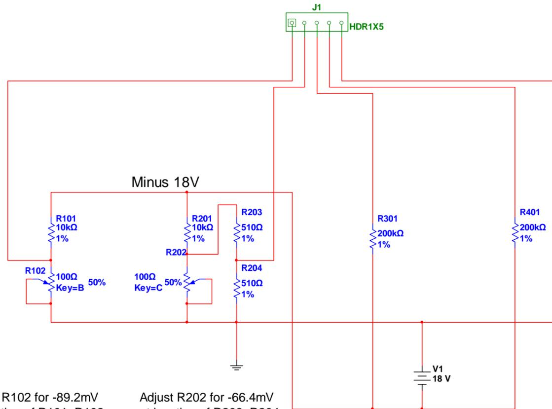
Adjust R102 for -89.2mV at junction of R101, R102 with the head attached.
