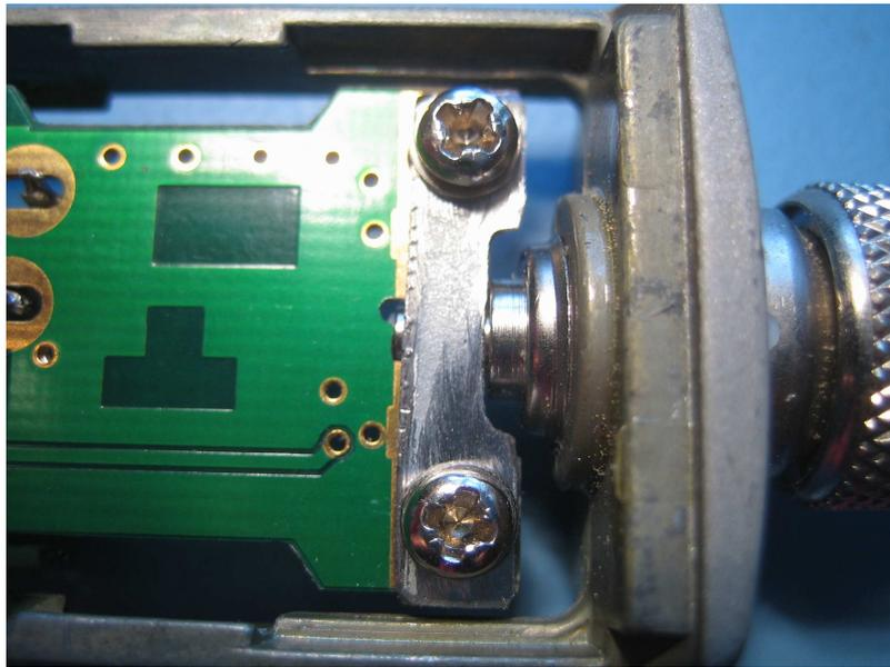
All that remains is to connect the 4 core cable to connection points 1 to 4, solder the input coax screen and use a fine wire to connect the centre core of the input coax to the pad next to R1, and finally to solder the centre connector of the output connector:
