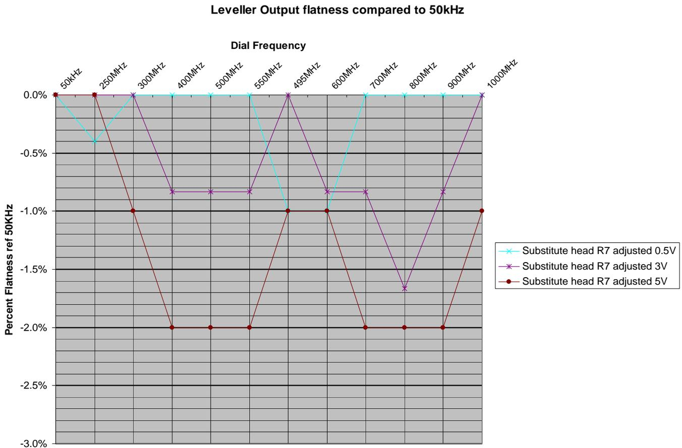
As you can see the worst case deviation of the output is [+0%, -2%] which is within the specifications of [+3%, -3%] as set by Tektronix, and only very marginally less good than my original head after I had adjusted the trim-pot.
